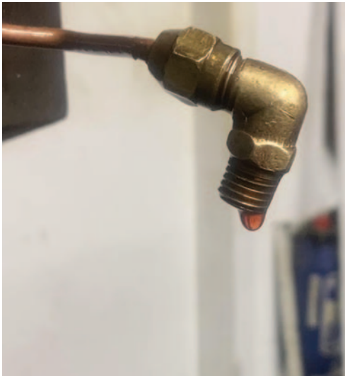
First drop of oil through the metering valve for a very long time!
