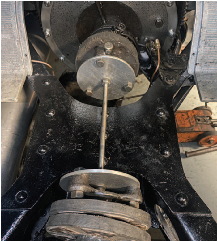
Clutch and gearbox refitted and aligned using bespoke (that means homemade!) aligning tool
